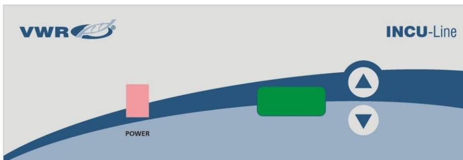
POWER - power switch: For turning the incubator ON and OFF. It lights when incubator is switched ON.
